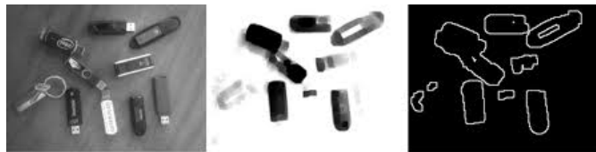
Fig -2: Image pre-processing step
