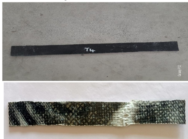
Fig-3.2 After tensile test
