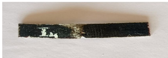
Before Impact Test
