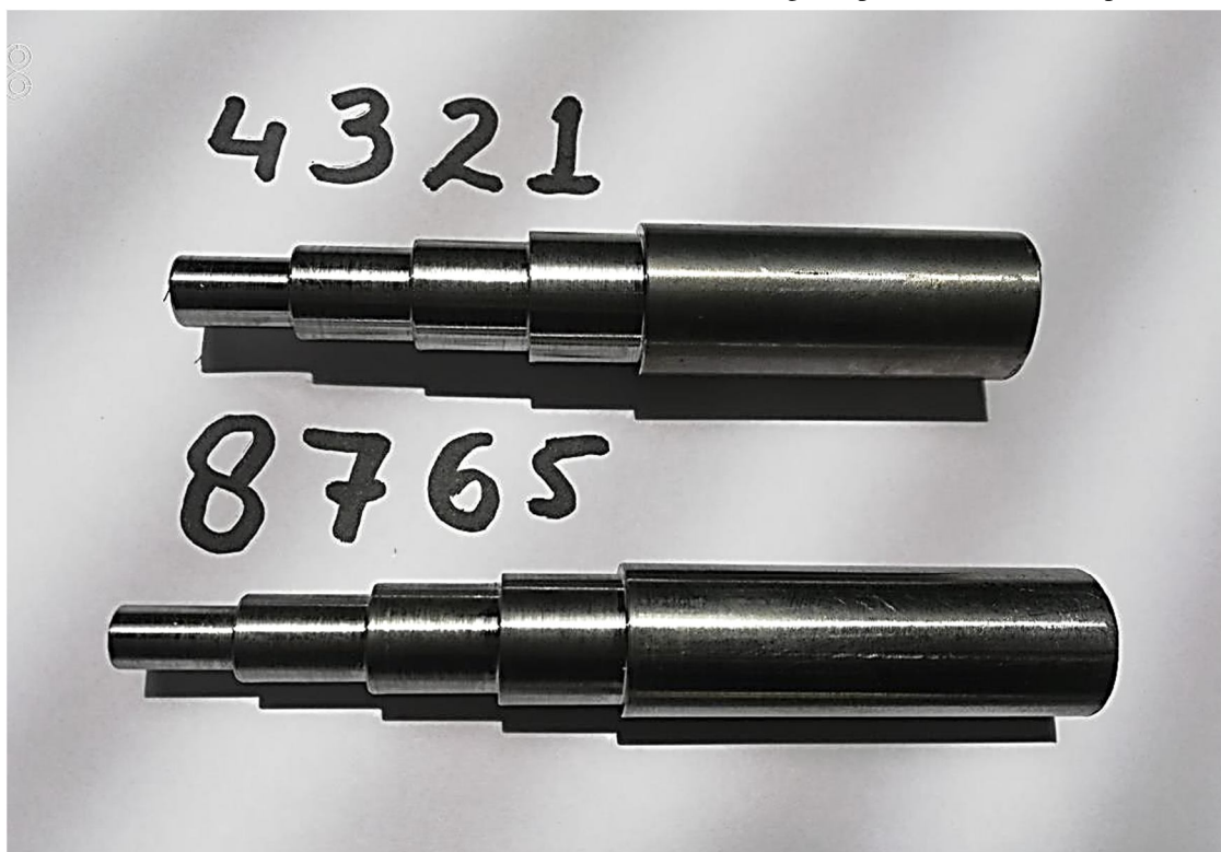
Fig. 16 Workpiece of titanium alloy (Ti-6Al-4V) after tuning
