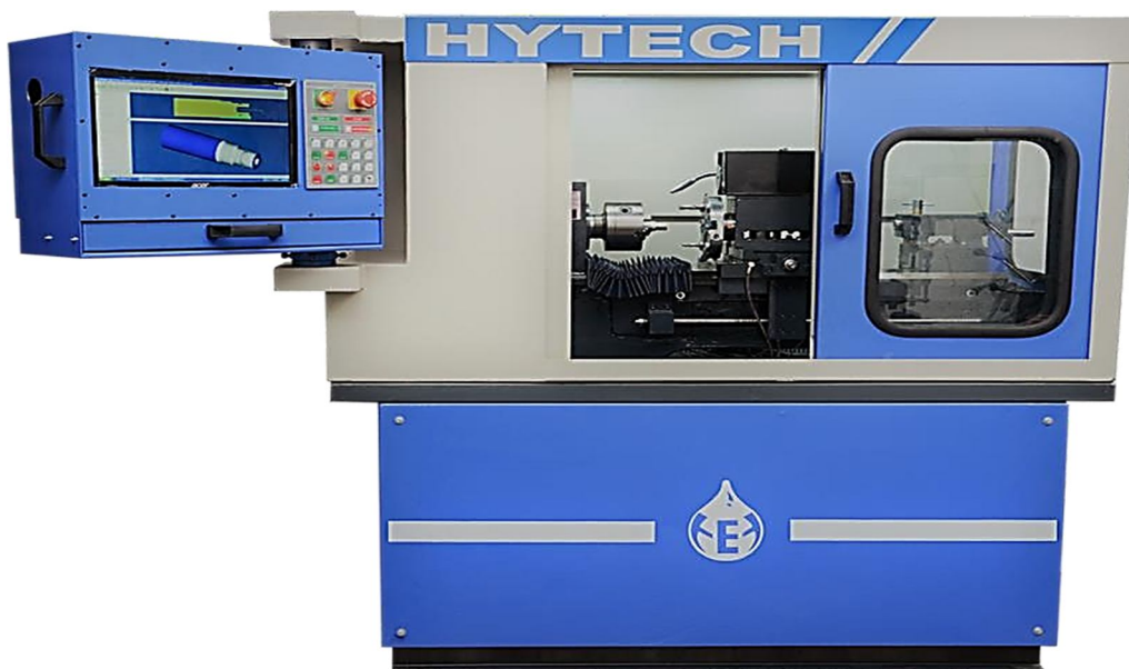
Fig. 6 HYTECH CNC trainer lathe machine
