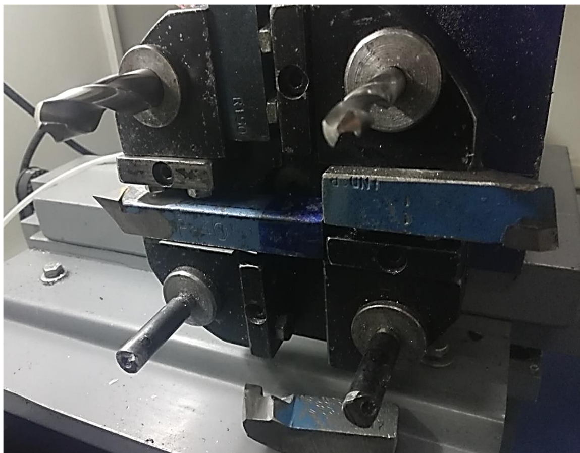
Fig. 9 Tungsten carbide tool with tool holder
