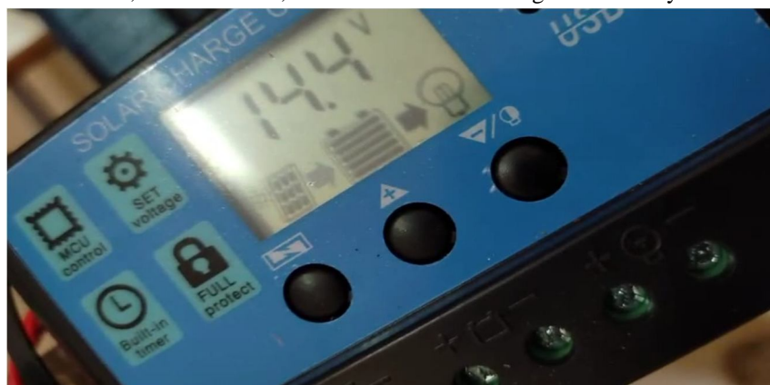
Fig 5.1: Reading from Charge Controller
