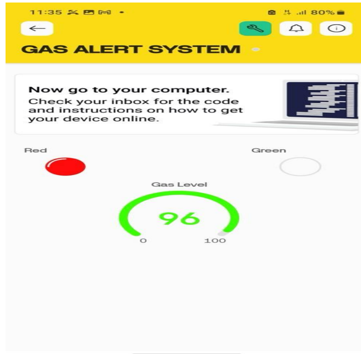
Fig. 8: Mobile application for the gas sensor reading
