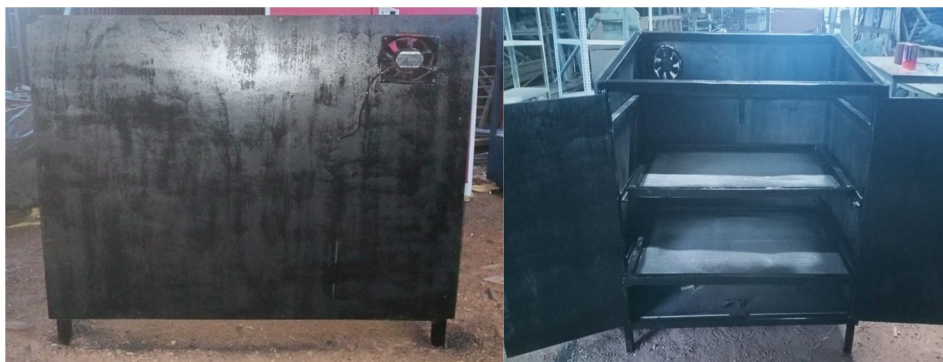
Fig 4.3 Working model of solar tray dryer
