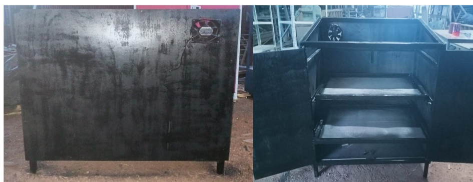
Fig 4.3 Working model of solar tray dryer
