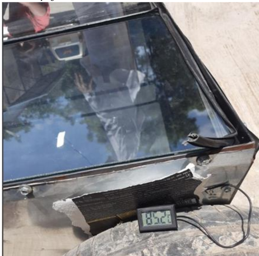
Fig. 16. Maximum achieved temperature in chamber
