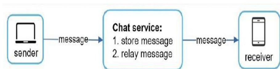
Figure 2. shows the relationships between clients (sender and receiver) and the chat service
