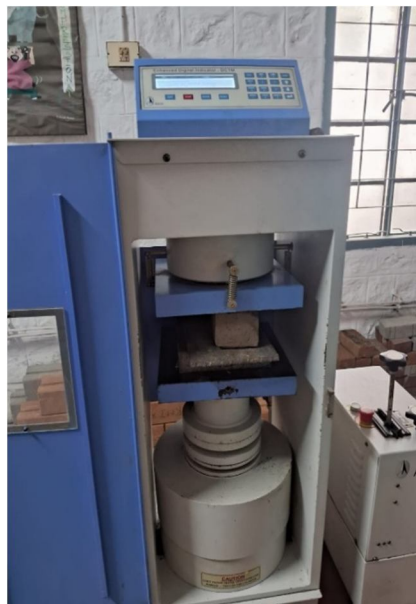
Compressive strength of conventional clay brick
