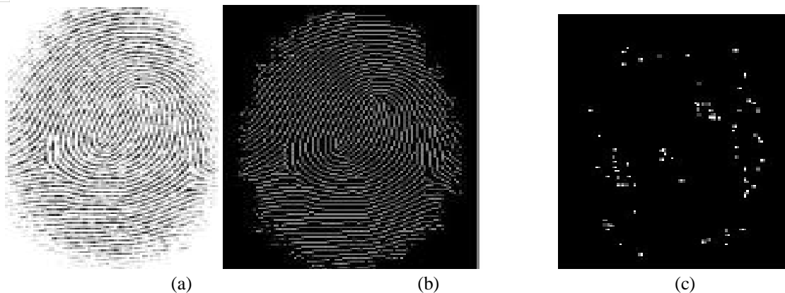
Fig 3.11: (a) Input fingerprint, (b) Thinned image, (c) extracted minutiae
