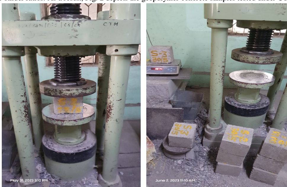
Fig. 2 Compression testing machine with geopolymer concrete samples
