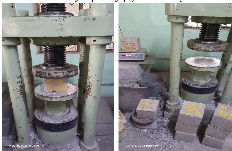
Fig. 2 Compression testing machine with geopolymer concrete samples
