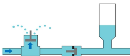
FIGURE 18: The automatic HRP working cycle.
