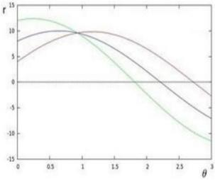
We see that the lines in Hough space intersect at  $\theta = 0.925$  and r = 9.6. Since a line in the Polar coordinate system is given by  $r = x\cos\theta + y\sin\theta$ , we can induce that a single line crossing through all these points is defined as  $9.6 = x\cos0.925 + y\sin0.925$ .
