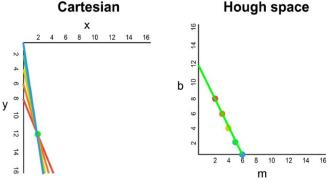
Whenever we see a series of points in a Cartesian coordinate system and know that these points are connected by some line, we can find the equation of that line by first plotting each point in the Cartesian coordinate system to the corresponding line in Hough space, then finding the point of intersection in Hough space. The point of intersection in Hough space represents the m and b values that pass consistently through all of the points in the series.
