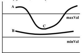
Edge A is higher than the maximum value so it is an edge. Edge B is between the maximum value and the minimum value, but it is not connected to any edge above the maximum value, so it is discarded. Edge C is between the maximum value and the minimum value and is connected to edge A, an edge above the maximum value. This means that C is an edge. For our pipeline, we first grayscale the image to reduce noise and then apply a 5 by 5 gaussian blur to decrease the amount of noise.
