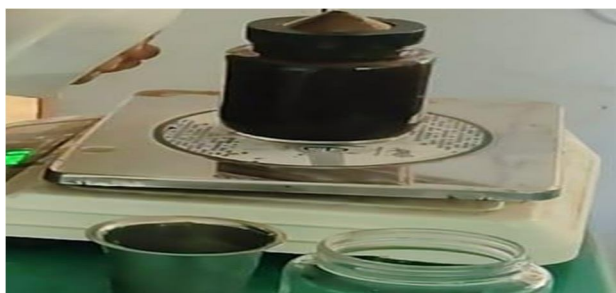
Fig 1 : Testing of specific gravity
