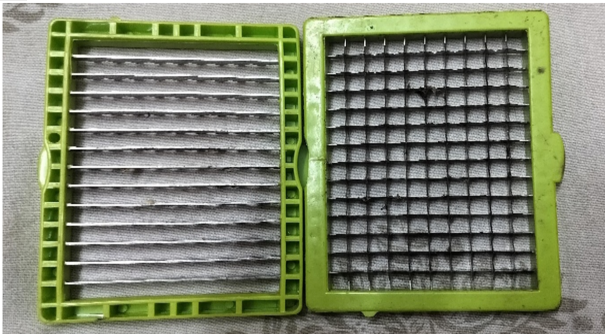
Figure 11: Different types of Blades used for cutting process
