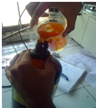
Figure 8: Pouring of mixture in separate container after stirring at constant temperature
