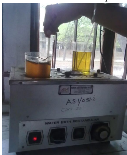
Figure 7: Stirring of Linseed oil and mixture for 30 min
