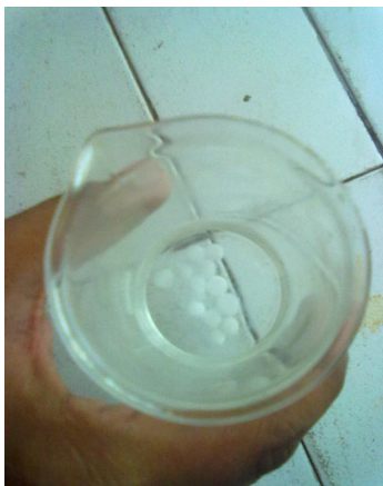
Figure 5: Mixing of KOH & methanol
