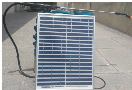
Fig.3 Fabricated solar pesticide sprayer (back sprayer)
