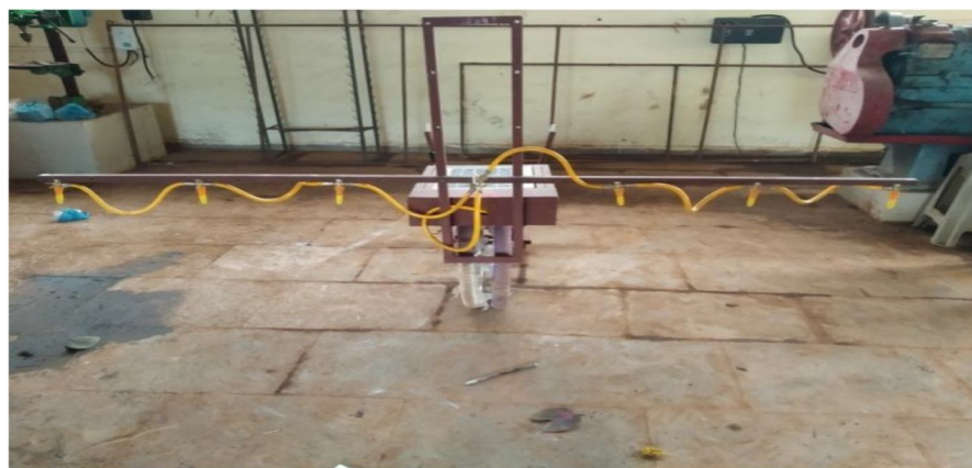
Fig.2 Solar operated trolley type sprayer
