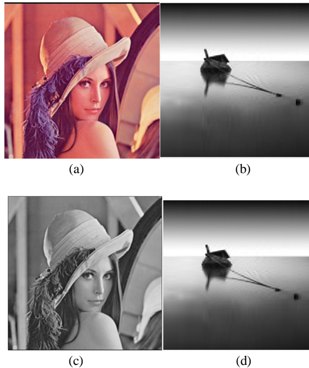
Fig. 4. Example of the proposed watermarking approach (a) The original image (b) The original watermark (c) The watermarked image (d) The extracted watermark
