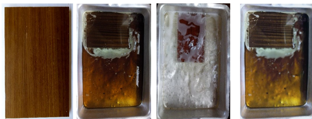
Fig.1 (a) Engineered wood floor (b) Boiling in linseed oil (c) Boiling in molten paraffin wax (d) Boiling in a mixture of linseed oil and molten paraffin wax
