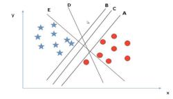
Hyper Plane C has a sufficient margin on the left as well as the right side, which makes it more robust for the new data points that might appear in the future. The output is generated by the activation function using a sigmoid kernel.
