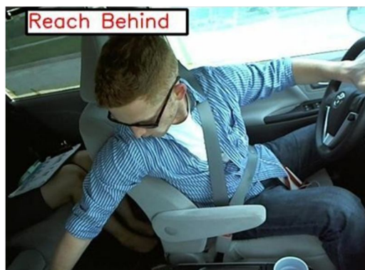
Fig.4 Driver detected while turning behind
