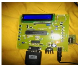
Figure(5) Over speed controller
