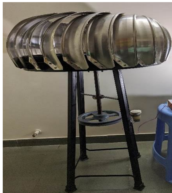
Fig. 2 Roof Ventilator with Pulley Arrangements
