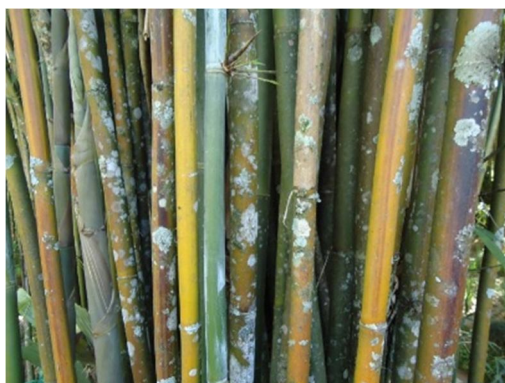
Fig. 3: Fungal degradation in bamboo [10]
