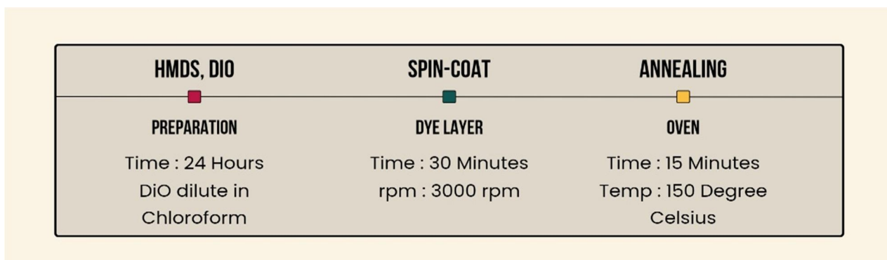
Figure 3 The process of dye deposition
