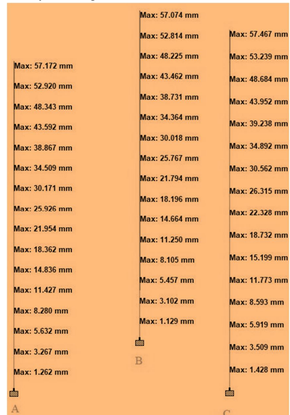
Figure 13. Displacement of Type B Building.
