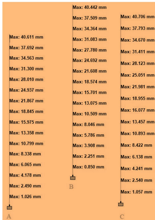
Figure 14. Displacement of Type C Building.
