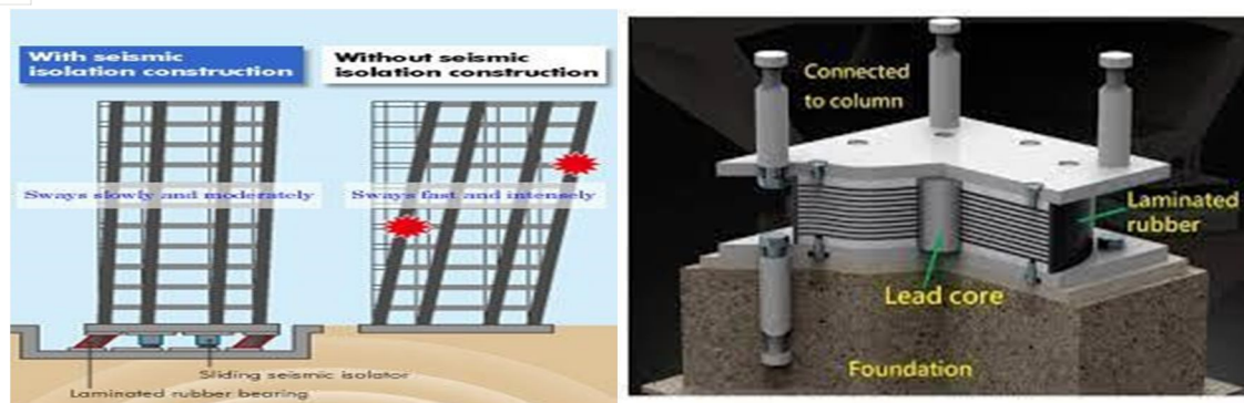
Fig.1 Isolation system and Lead rubber bearing
