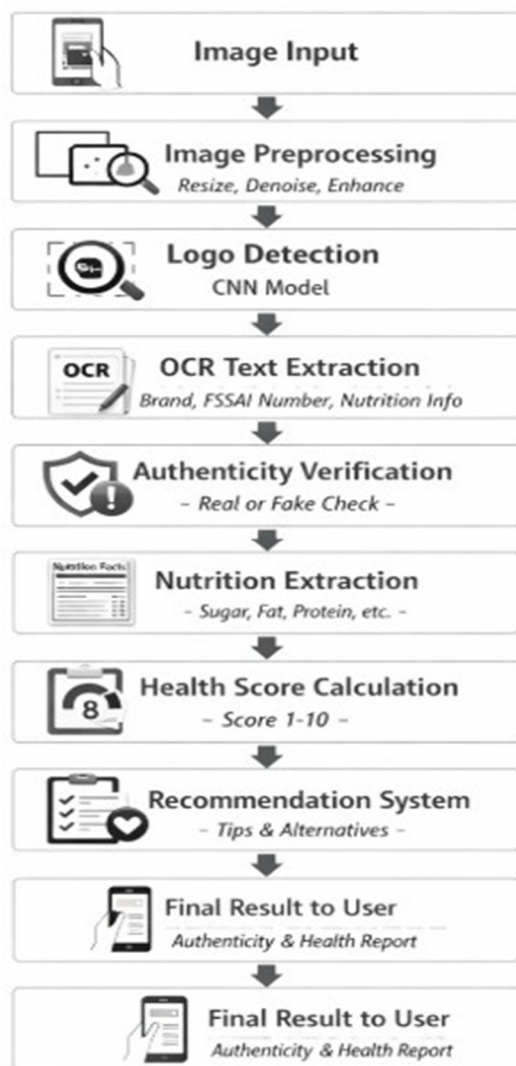
Fig. 1. EatSafe system pipeline: from image input to authenticity verification and nutrition report.
