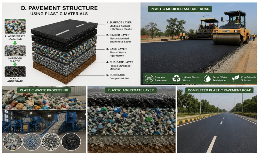
Fig. III. D. 1. Flexible Pavement
