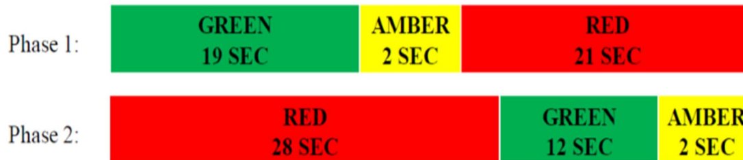
Fig 11: Signal Phase Diagram for peak hours
