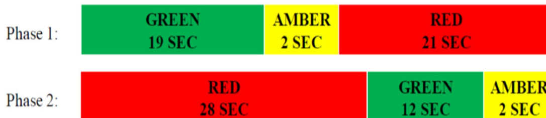
Fig 11: Signal Phase Diagram for peak hours
