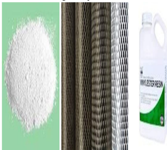
Figure 1.2: AA6061 (Aluminum Alloy 6061) powder b) basalt fiber mat c) vinyl ester resin.
