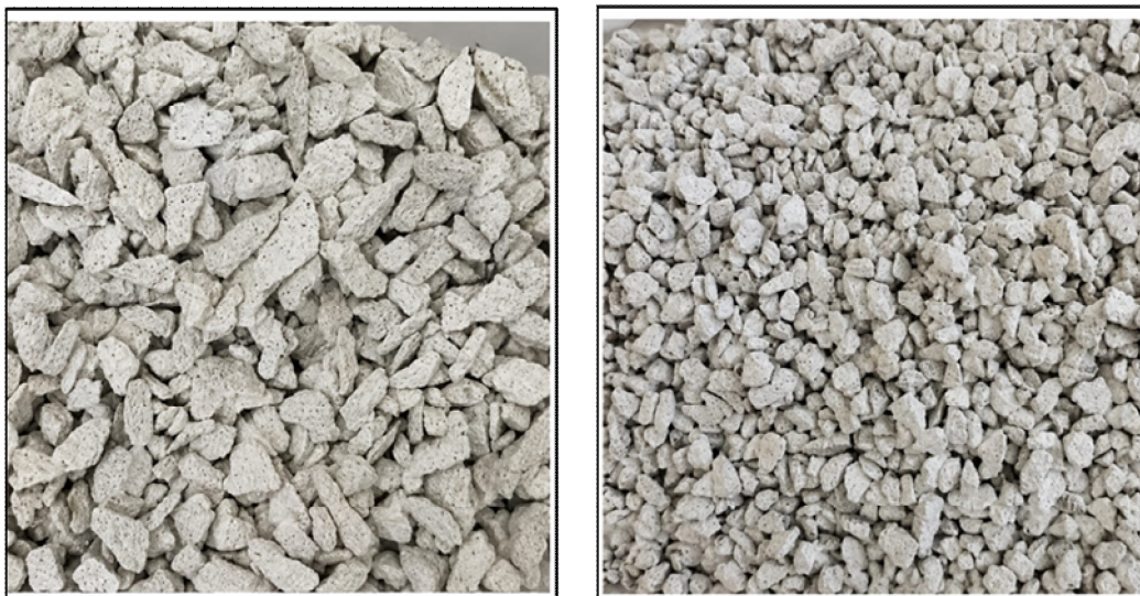
Fig. 1. Recycled concrete aggregate obtained from demolition waste
