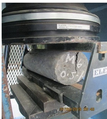
Fig 4 Split tensile strength testing of cylinder specimen
