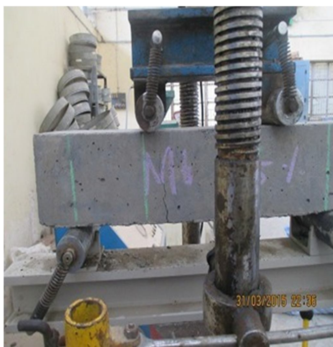
Fig 6 Flexural strength testing of beam specimen
