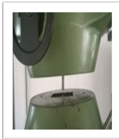
Fig 19: Piece in the wake of breaking in UTM
