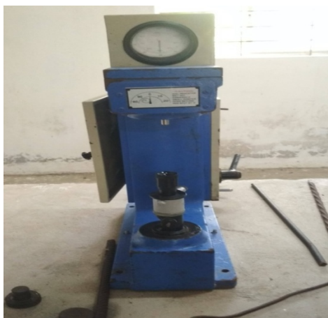
Fig 24: Brinell and Rockwell Hardness Testing machine
