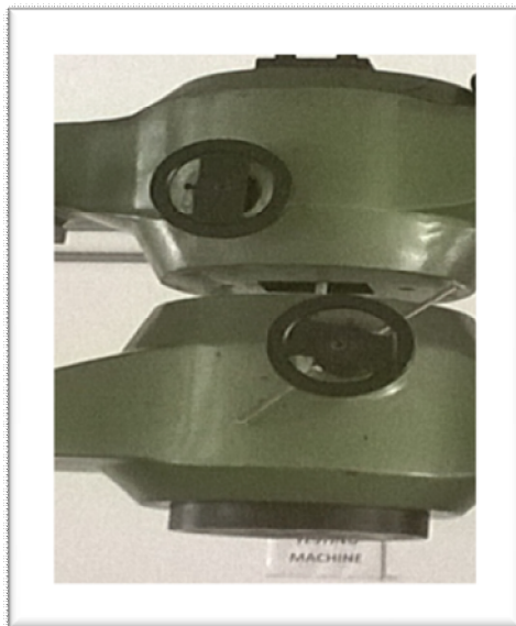
Fig 18: Piece before breaking in UTM
