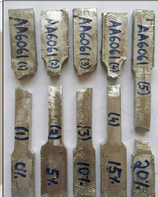
Fig 17: Tensile Tested Pieces
