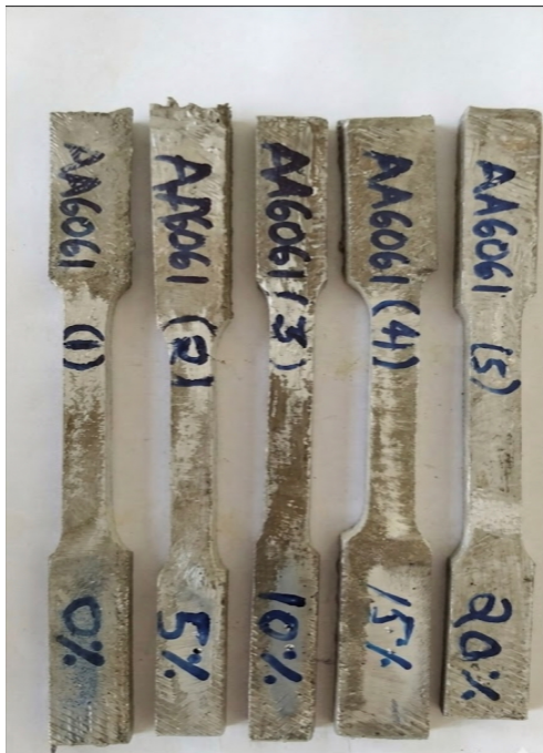
Fig 16: Al Cast Alloy in sync with ASTM E8 Standards
