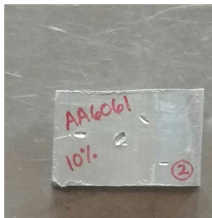
Fig 25: Brinell hardness tested pieces
