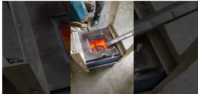
Fig 4 stir casting process
