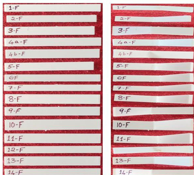
Fig. 8: Sample before and after the flexural test
