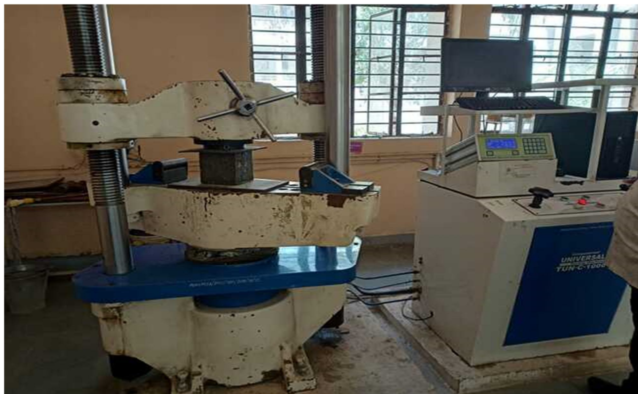
Fig. 5 Compression test on hardened blocks
