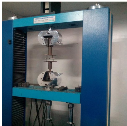
Fig. 4 Cross lap joint tensile testing
