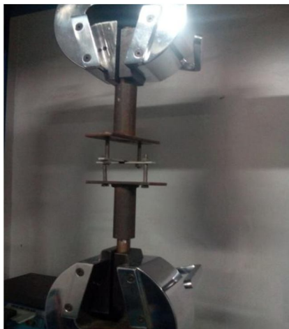
Fig. 2 Fixture for clamping of Cross lap joint in Universal Testing Machine
