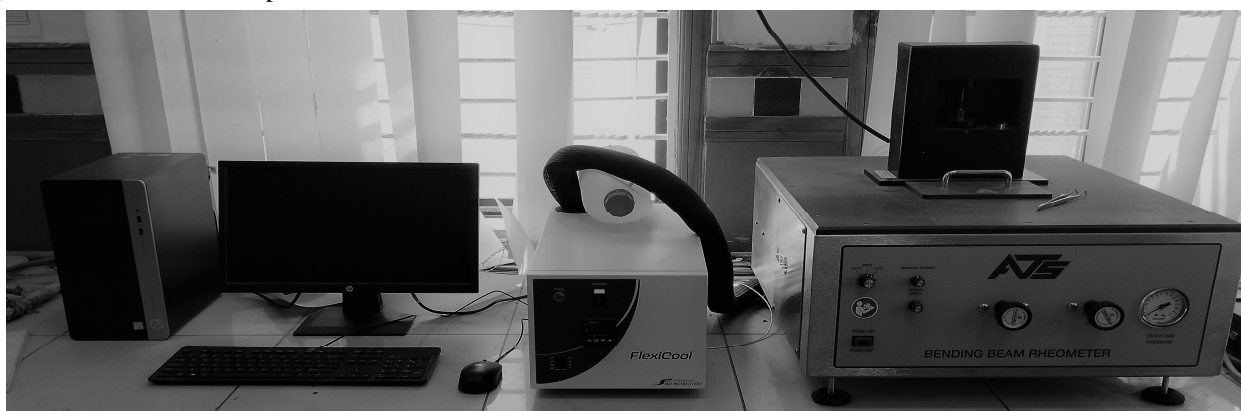
Figure 5 : Bending Beam Rheometer (BBR)
