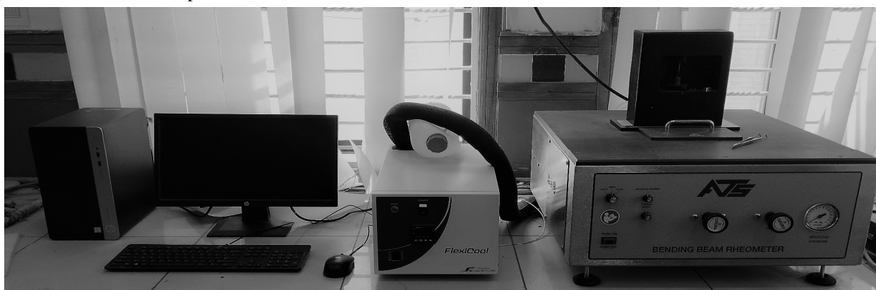
Figure 5 : Bending Beam Rheometer (BBR)
