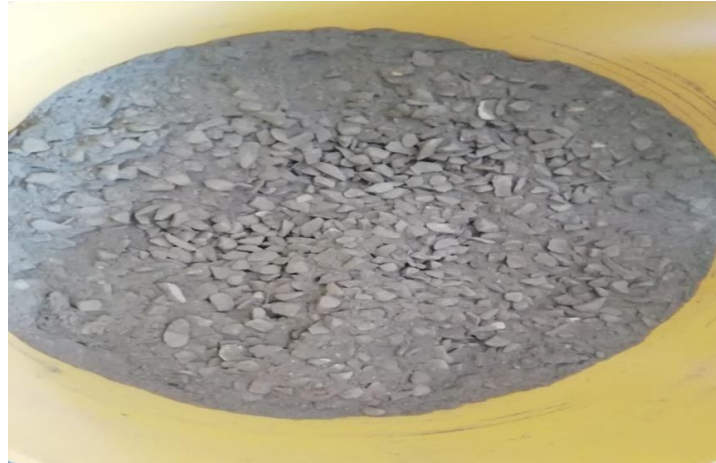
Fig. 3 Dry mix of concrete mix
