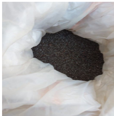
Fig. 1 Fine Metal swarf
