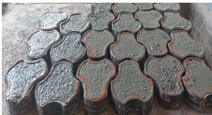
Fig. 5 casting of samples
