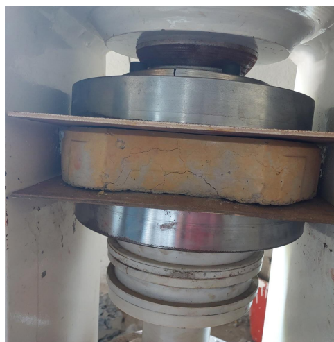
Fig. 7 Testing of sample in CTM
