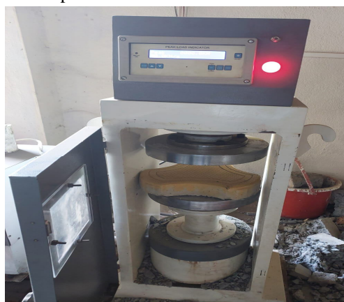
Fig. 6 Compression Testing Machine
