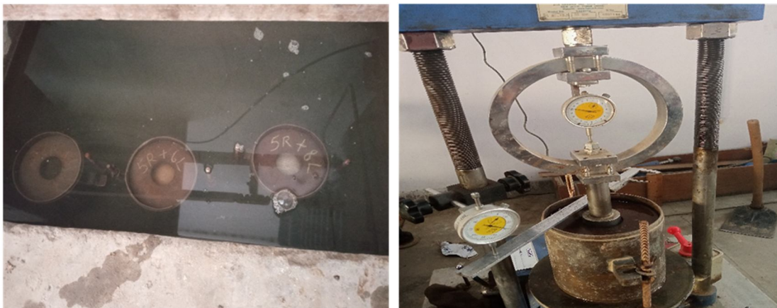
Fig. 4 CBR Soaked sample and CBR machine
