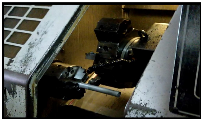
Fig.1.4 Machining of compression specimen
