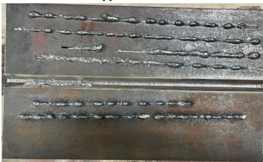
Fig.10 Bead on Plate - Top Angle View
