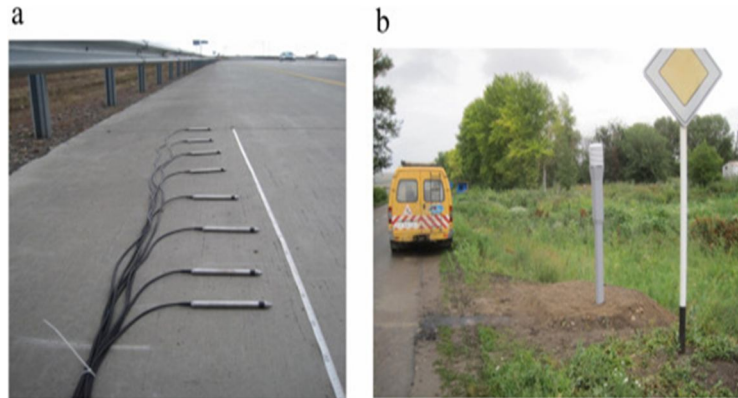
Figure No. 4 Technical systems for temperature and moisture measurement's a– one set of temperature and moisture sensors; b – surface measurement part.
