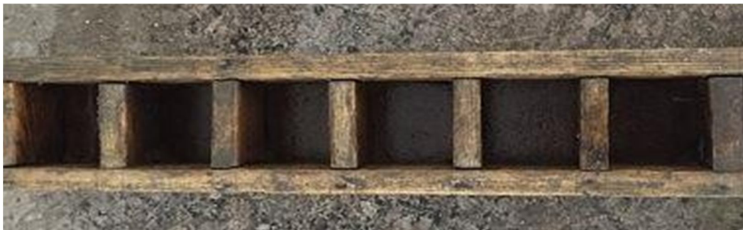
Fig 2: Moulds of Cubes of Size 50mm*50mm*50mm
