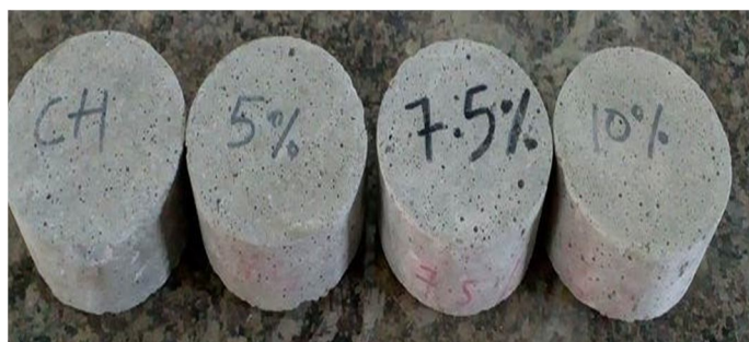
Fig 9: Cylindrical Slices (100mm diameter and 50mm height)
