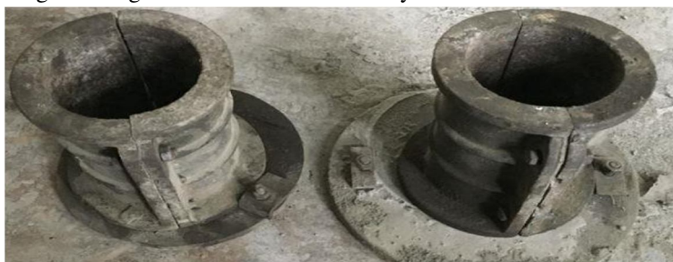
Fig 8: Moulds of Cylinder of 100mm dia. and 200mm height
