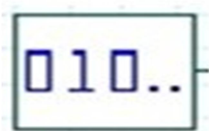
Figure 18 PRBS generator symbol
