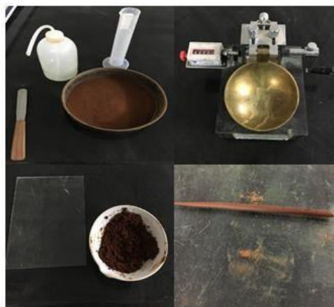
Figure 3.1 Images of the LL and PL test
