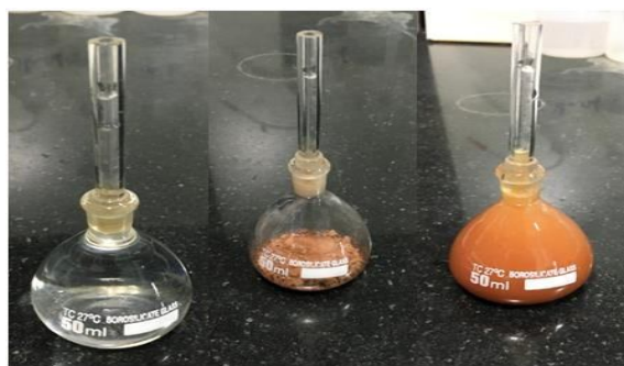
Figure 3.3 Specific gravity test by density bottle method
