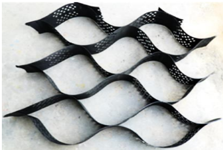
Figure 3.6 Typical geocell used in the study
