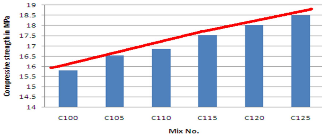
Fig. 8 – 14 days compressive strength of C1 (ordinary Portland cement)category mix
