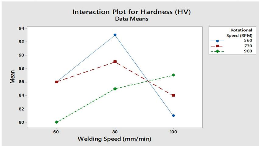
Fig 5.9 Interaction effects of rotational speed & welding speed on hardness
