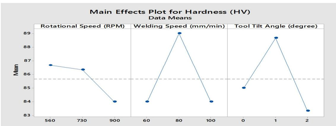
Fig 5.3 Main effects plot for Hardness (HV)
