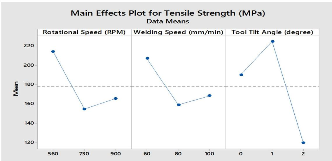
Fig 5.2 Main effects plot for Tensile strength (MPa)
