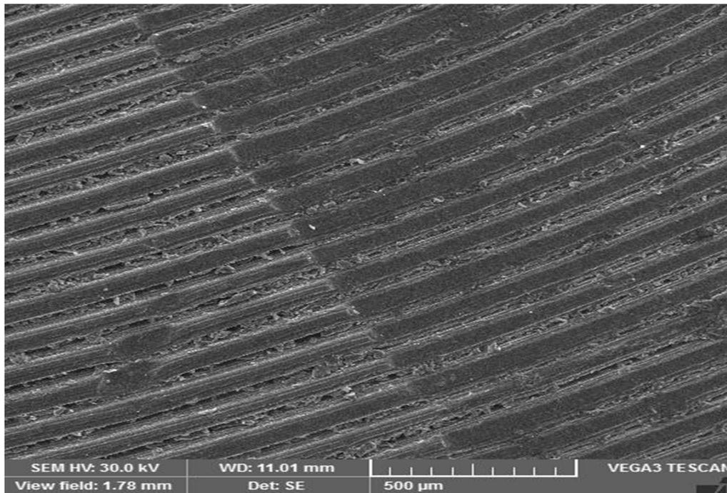
Fig 4.5 Microstructures of SZ of FS welded joint
