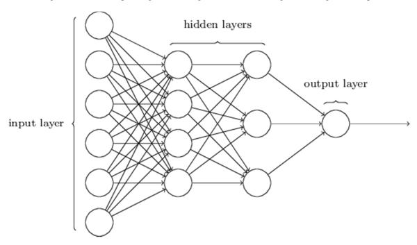
As discussed earlier here, each sentence is broken down into individual words, and each word is then used as input for the neural networks. The weighted connections are then calculated by different iterations through the training data thousands of times, each time improving the weights to make it accurate.
