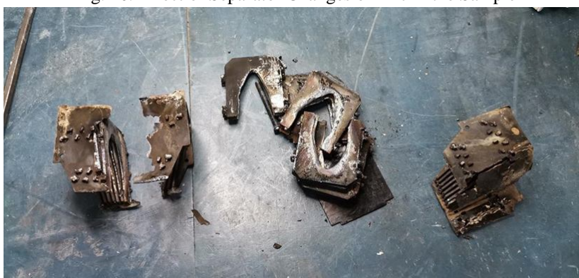
Fig. 11. Sample Separator Deformation
