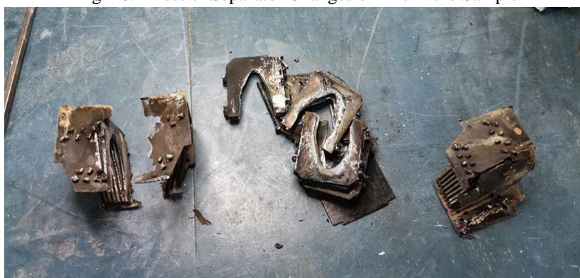
Fig. 11. Sample Separator Deformation
