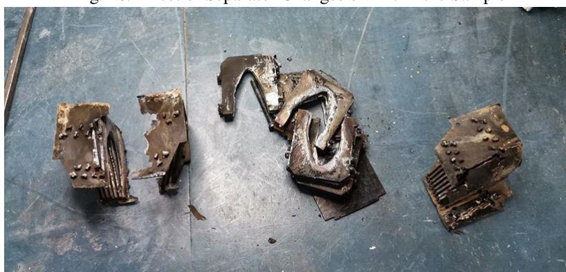
Fig. 11. Sample Separator Deformation
