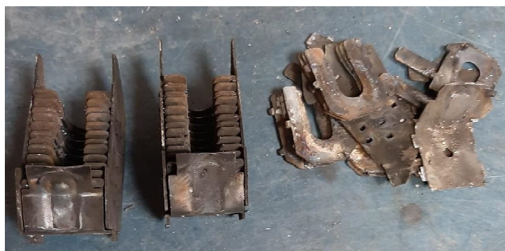
Fig. 5. Damage in Separators of Non-Limiter Circuit Breakers
