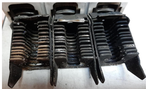
Fig. 7. Damage in Separators of Limiter-Equipped Circuit Breakers
