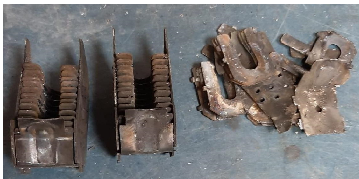
Fig. 5. Damage in Separators of Non-Limiter Circuit Breakers
